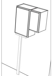
If you are working alone, improvise a T-support from two sections of 2x4. Pad with carpet scraps or soft cloth to prevent scratches. Use this to prop the front side of the cabinet to the proper height while you install screws.
