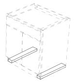
For peninsula or island installation, trace the cabinet footprint on the floor and secure blocks to floor along this line under the cabinet. Fasten the cabinet to the blocks.
