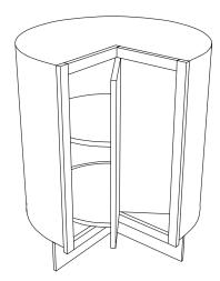
Just one lazy susan base (block 3320) doesn't have side or end panels. To support the countertop in a corner above this lazy susan base, attach strips of 1x2 to the wall and level with the height of the cabinet tops, as shown below.
