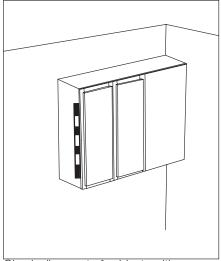
Check alignment of cabinets with a carpenter's level on front, sides and bottom.
