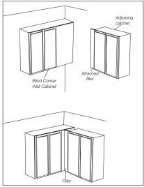
Tip: For a custom fit, you can adjust blind corner cabinets in both directions. First, install the corner cabinet and all other wall cabinets on the same wall. Next, cut filler to width and length as needed in the same manner as described for attaching one unit to the next. Last, install adjoining cabinet with filler attached.
