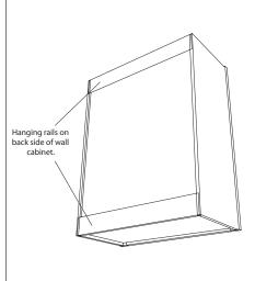
Use at least two #8 x 21/2" screws through the hanging rail of the cabinet. Attach only loosely at first, to allow for necessary adjustments.
